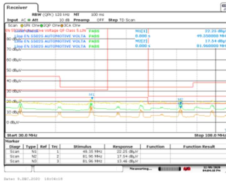
Figure 4. Isolated 5-V reference design (with interleaving layers) conducted emissions versus CISPR 25 Class 5, 30 to 108 MHz: passed with 4.5 dB of margin, with the worst case being a “CISPR average” detection at 82 MHz. Source: Texas Instruments
