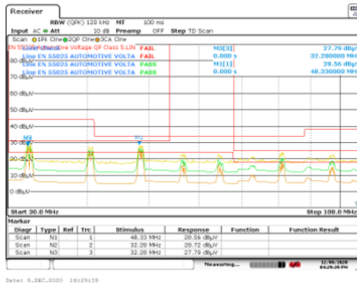
Figure 5. Unreleased board (no interleaving layers) conducted emissions versus CISPR 25 Class 5, 30 to 108 MHz: failed by 3.8 dB of margin, with the worst case being a CISPR average detection at 32 MHz. Source: Texas Instruments
