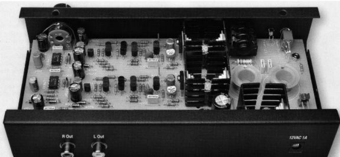
The PCB assembly is a neat fit inside the recommended Altronics case. Note how the body of the volume control pot (top, left) is earthed using a length of tinned copper wire. This wire is looped across the top of the pot's body and is terminated in solder pads on either side (see Fig.9).
