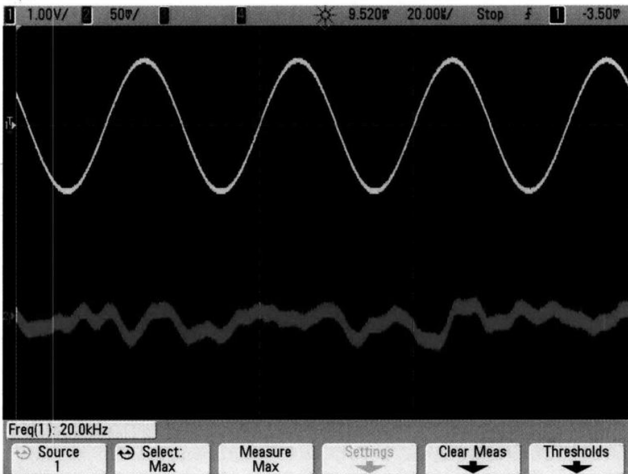
Fig.8: the green trace in this scope grab shows the distortion residual for 100mW into 32Ω at 20kHz. Most of this is actually noise with very little harmonic content. Into lower load impedances (eg, 8Ω) the distortion becomes more apparent and is primarily third harmonic, with some higher harmonics.
